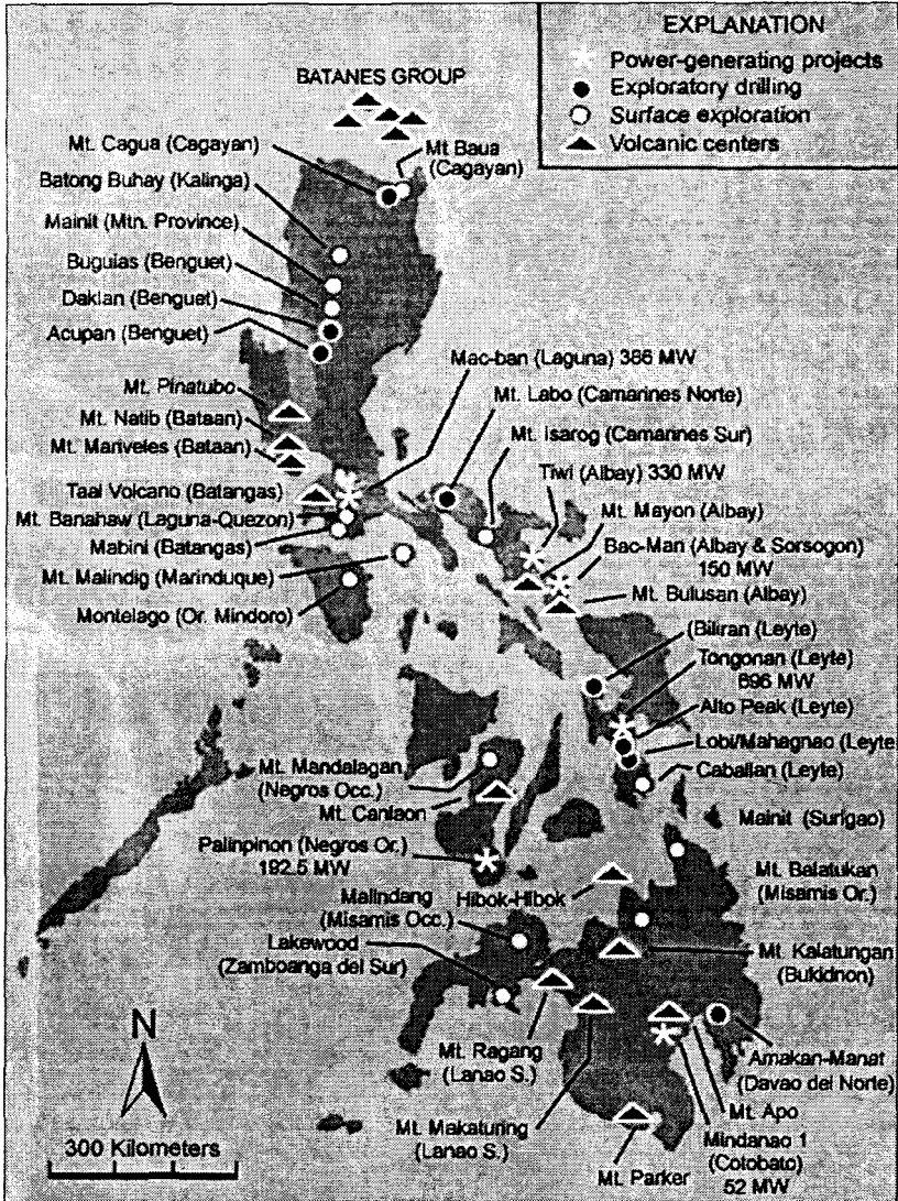
FIGURE 13. Major Philippine geothermal energy sites. Modified from PHIVOLCS data.
